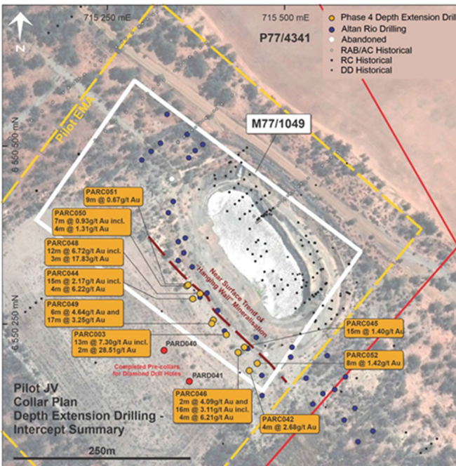
Left – Figure 1: Pilot Project, Collar Location and Phase 4 Drill Intercept Summary Above – Figure 2: Longitudinal Section
